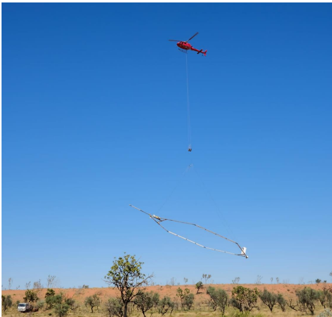
Figure 1: Helicopter-borne SkyTEM system operating at Paterson North
